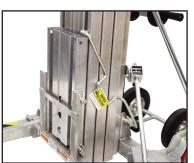
Mast hold bar for horizontal transportation. Hold down bar can be reshaped if bent.
