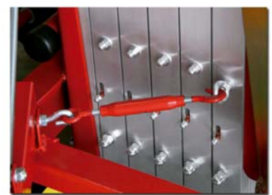
Adjustable mast blocking system for horizontal transportation.
