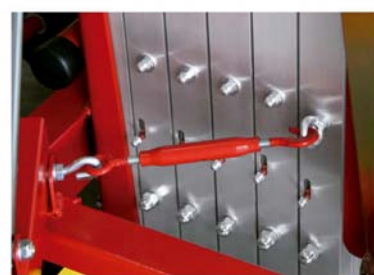
Adjustable mast blocking system for horizontal transportation.
