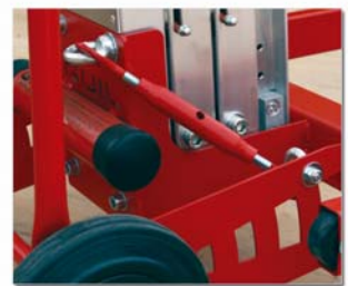
Adjustable mast blocking system for horizontal transportation.
