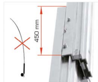
More mast overlap. Prevents fishing rod effect
